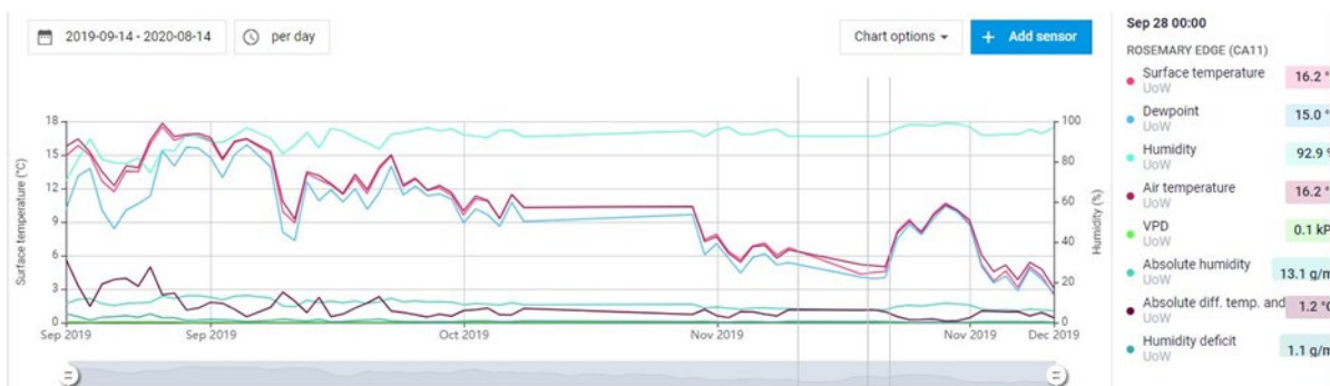
Figure 45. A screen shot from the Rosemary trial in the nursery glasshouse, showing the records of humidity (pale blue upper line) and air temperature (dark pink line) from inside a Zensie screen over three months. Leaf surface temperature (red line) from an arm probe close to a leaf surface at times differed from the air temperature. Values of dew point, vapour pressure deficit (VPD), absolute humidity and humidity deficit are calculated by the system.
